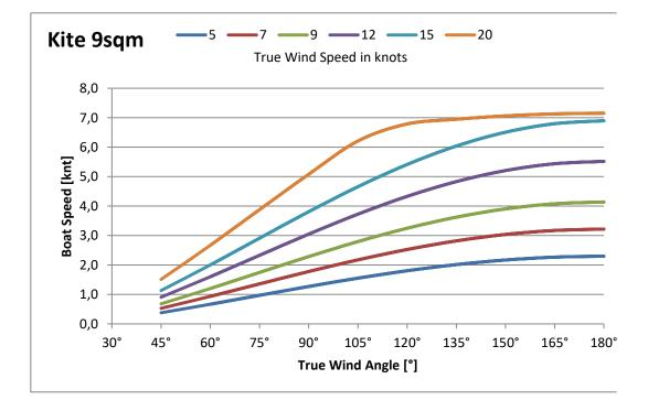
\* Values are based on the drag of a standard displacement hull with fin keel. The results are aproximated values. This information is supplied without liability and under terms of nondisclosure.
